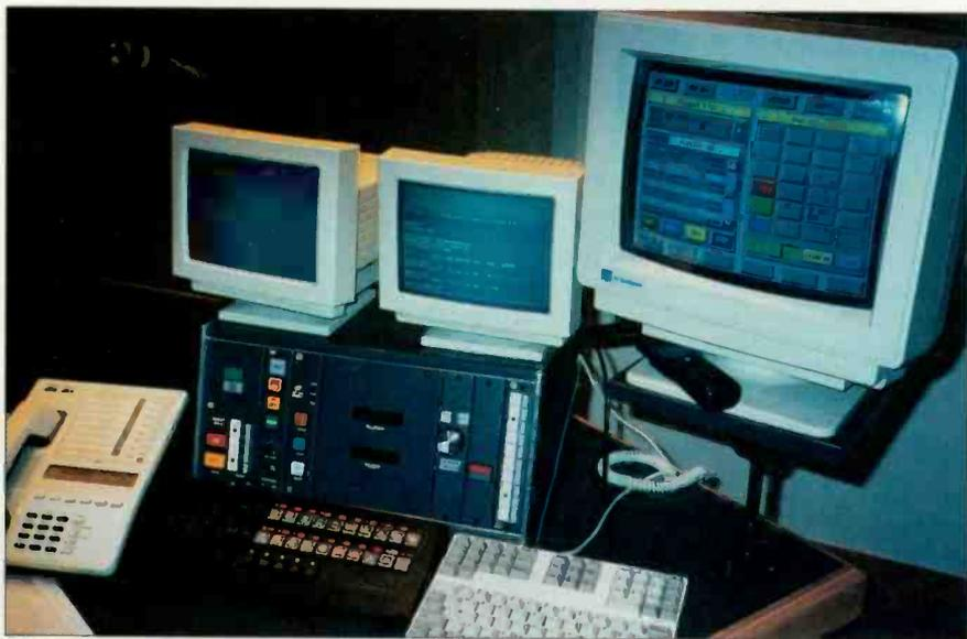
At WMC-AM in Memphis, an ENCO Systems' DAD486x network is used for live-assist daytime operation and overnight automation of the station's news/talk format. Seven DAD486x workstations and two file servers are linked via LAN, with separate monitors used for audio (touchscreen at right) and text (at center) displays. In this talk studio, a third monitor (at left) displays queued caller data.
