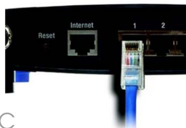
**D** Repeat step C to connect additional PCs or other network devices to the Router.
