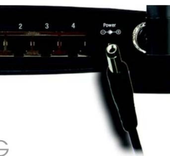
**IMPORTANT:** Make sure you use the power adapter that is supplied with the Router. Use of a different power adapter could damage the Router.
